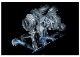
TwinScroll turbocharger with a cross-bank exhaust manifold: the exhaust flows from each of two cylinder pairs with a 360° firing interval are combined and routed along separate channels before reaching the turbine wheels of the turbochargers. This guarantees that gas flow is not compromised. It's a highly efficient charging concept that leads to optimum energy transfer – and, therefore, extremely spontaneous reponsiveness.
