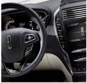
Innovative signature shifter: The MKC Concept's distinctive pushbutton gear shift selector optimizes space by eliminating the bulky traditional console shifter. It also increases console stowage space.
